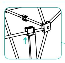
a. Slide top brackets onto X bars on frame.
