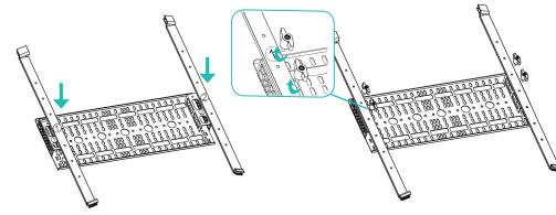
**b.** Place support struts in desired location on mount. (Match #'s on struts with mounting plate. Struts are also marked top & bottom)
