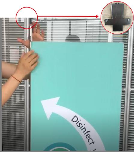
Insert connector into the hole on the top corner of the frame
